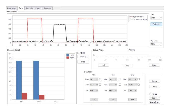
② Calculate the phase difference between the phase of the antenna and the phase of the surrounding equipment:Left-click the phase of the antenna (the far right edge of the red box)
