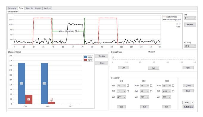
③ Enter the acquired phase difference value into the "Phase" field in "Parameter Settings", and then click the "Set" and "Save" buttons. Note: When the phase difference we acquired is 59.4, then, we can simply take the integer of portion to input 60.
